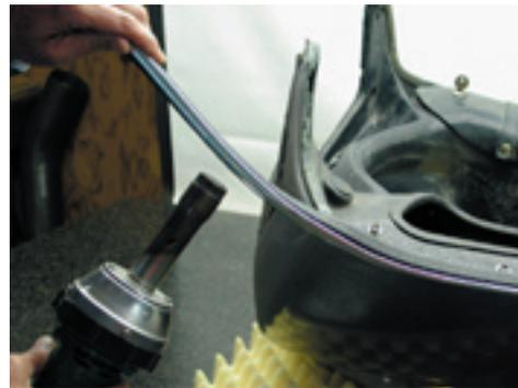
2) Test fit new edging and bend edging to shape. Begin on the long, straight section. Leave 2" at each end.
