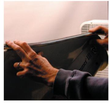
**Paint the Hotcha Glue on both and fit edging onto fairing. Put into place.**
